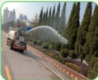
Recycling rainwater for greening and dustfall
