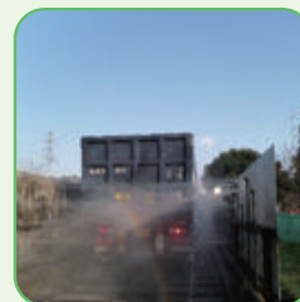
Truck washing at the side door of the raw material
